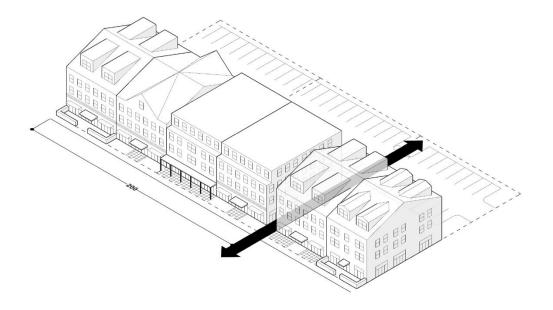
2. When provided, pedestrian passages may be designed as an open-air passage between buildings, a covered atrium providing continuous protection from the elements, or as an up to two (2) story passage through a building.
