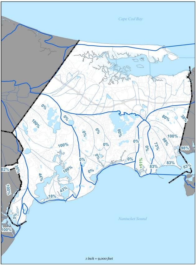
Figure 2-10: MEP Modeled Future Target Septic Load Removal
